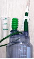
**Picture 2** (far left) shows the green concertina-like valve fully contracted, which shows maximum vacuum or suction.
